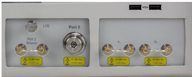
Front Panel: 'Normal' (left) and 'Reversed' (right) Configurations
